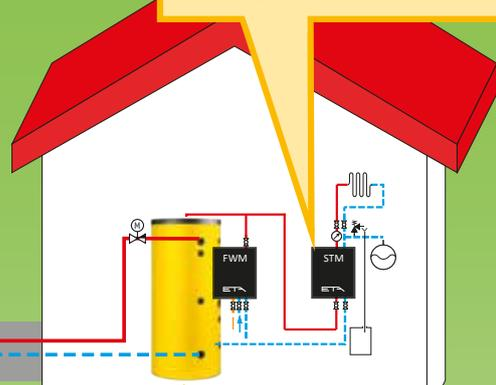
In that way hot water is economically, hygienically and quickly prepared using the **ETA ECO tank** and the **ETA fresh water module**.
