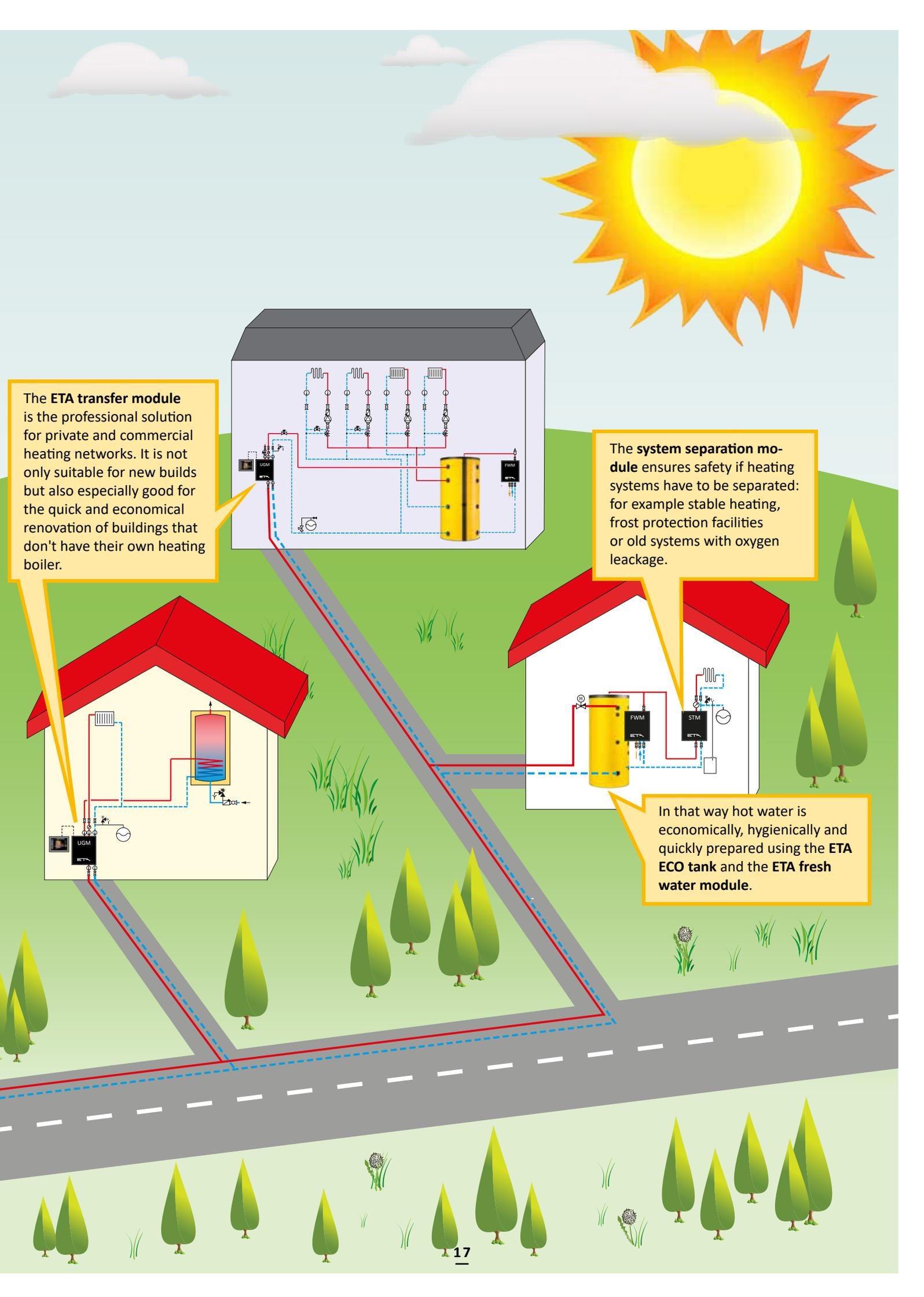
The **ETA transfer module** is the professional solution for private and commercial heating networks. It is not only suitable for new builds but also especially good for the quick and economical renovation of buildings that don't have their own heating boiler.
