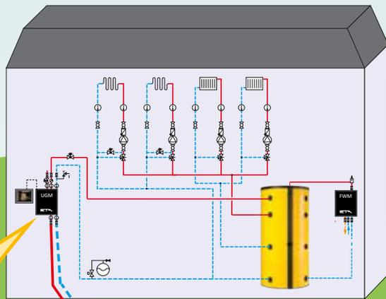
The **system separation module** ensures safety if heating systems have to be separated: for example stable heating, frost protection facilities or old systems with oxygen leakage.
