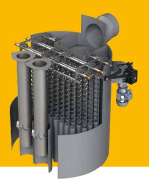
Permanent de-ashing The moving grate and ash rake are driven by just one motor. The stoking interval of the rake is fully automatically adapted to the requirements - and from the residual fuel that the lambda probe measures, the combustion chamber temperature and the relevant required output. So grate de-ashing takes place permanently. The system therefore does not need to be switched during ash removal.
