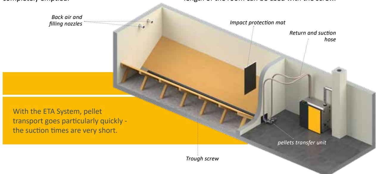
With the ETA System, pellet transport goes particularly quickly - the suction times are very short.
