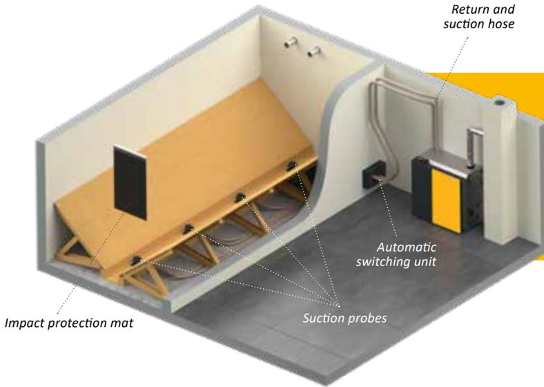
With the suction probes, nearly any room can be used as a pellet store, even if the store room is angular. Eight probes are also possible with larger store rooms.
