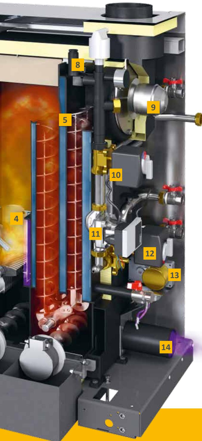
**8 Safety devices:** A safety valve and an electronic pressure sensor protect the boiler from overpressure. An automatic bleed valve is also integrated, so unwanted air is removed from the water circuit. The boiler does not need a thermal emergency cooling valve, as there is never too much fuel in the boiler that could cause overheating.
