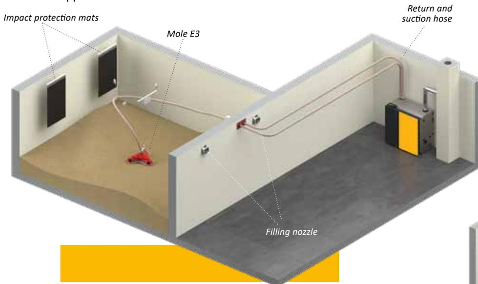
With the E3 mole conveying system, the storage space can be almost completely emptied and the sloping wooden structure is eliminated.
